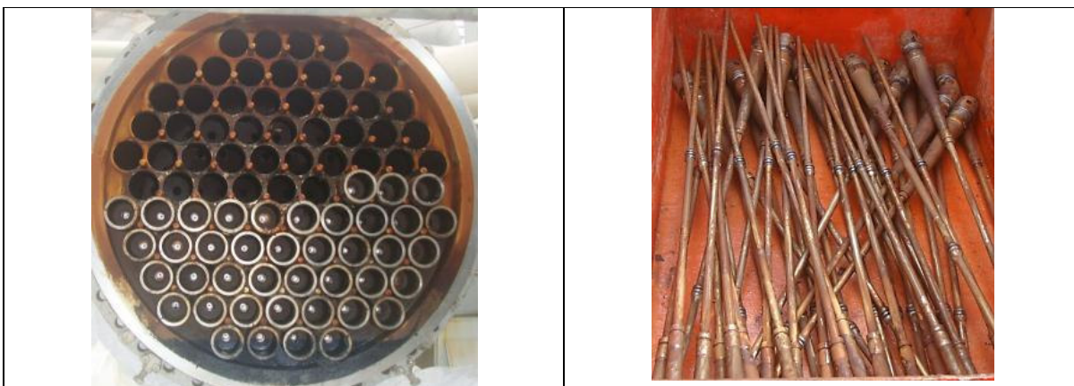
Figure 13. Hydrocyclone interior after long-term application with CaN inhibitor formulation at the facility from Field B.
