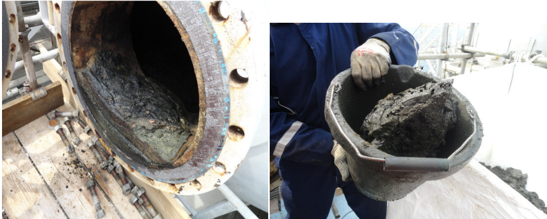
Figure 2. Field B facility. Images showing CaN solid removed from the Coalescer vessel.
